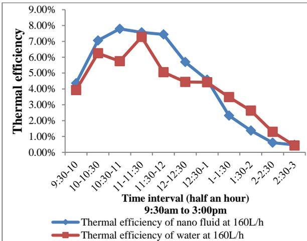
Figure. 7 variations in thermal efficiency with respect to time
