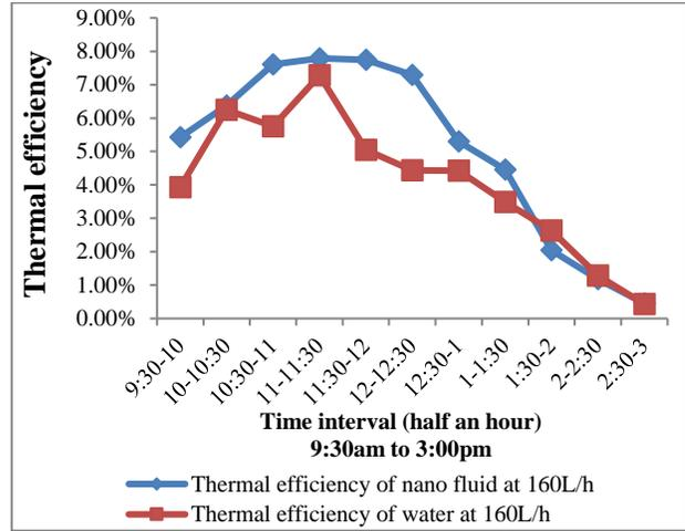
Figure. 9 variations in thermal efficiency with respect to time
