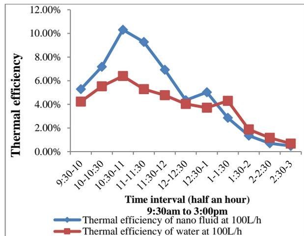
Figure. 10 variations in thermal efficiency with respect to time
